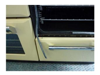
THE DOOR SEAL IS REMOVED BY JUST PULLING IT IS SECURED IN THE GAP BETWEEN THE CAVITY AND FRONTFRAME AND REQUIRES NO OTHER FIXING
