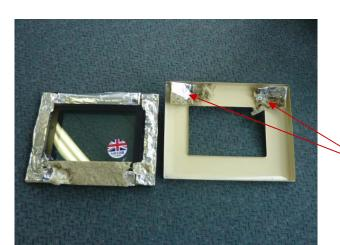
WITH THE SECURING SCREWS REMOVED THE INNER PANEL CAN NOW BE SEPARATED FROM THE OUTER PANEL
